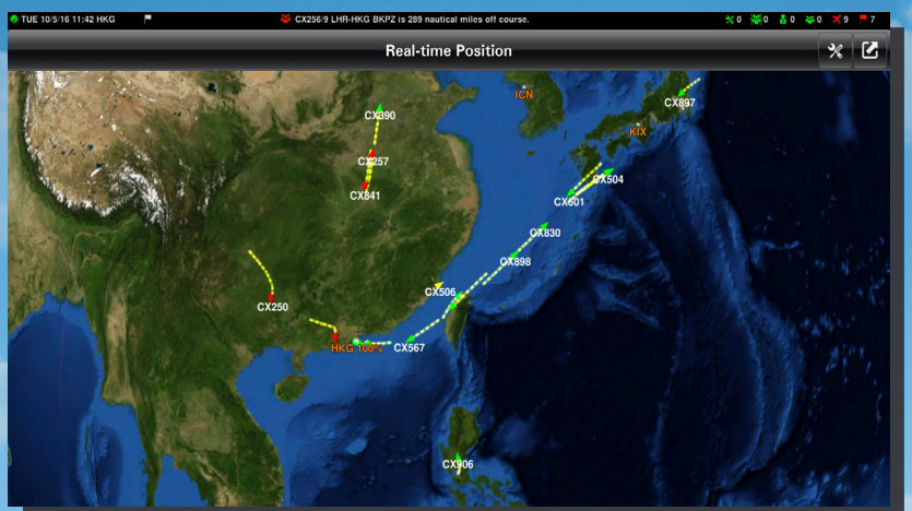
Fig 3. Globe with aircraft positional data and off course alerting
